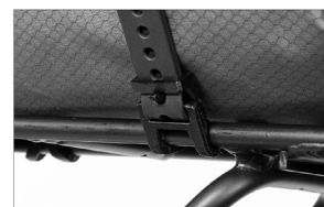
Detailed view of rack straps mounted on the luggage carrier
